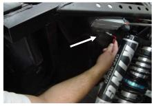
Secure the back of the box using the provided Allen screws and washers the Allen head goes toward the outside of the vehicle so the nut is inside the enclosure
