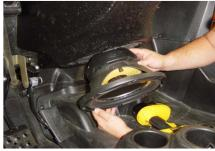
After the enclosure is mounted, pull any remaining speaker wire under the dash and mount the speaker in the box.
