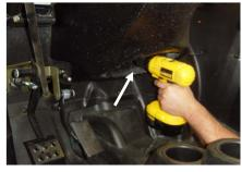
Once the enclosure is hung with the U-bolts,  $\operatorname{Pre}$  drill the mounting holes in the back of the box toward the firewall
