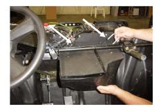
We recommend Pre drilling the holes using a 1/8" drill bit to make screwing in the subwoofer easier. Drill a 1/4" hole in the lower top of the box to run the speaker wire out of the enclosure. **NOTE: Sealing this hole to prevent air leaking will improve sound quality**
